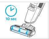
**5.** Brush roll starts spinning. Brush roll will not spin when machine is upright. The solution may take up to 10 seconds to fully wet brush roll.
