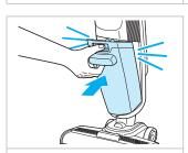
7. Insert bottom of tank first. Pivot top toward the machine until it clicks.
