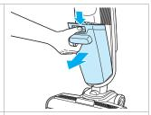
**3.** Press button on top of dirty water tank, grab front handle and pull out.
