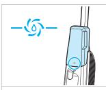
1. Make sure water reaches the clean-out cycle line on clean water tank. Refill with water if needed.
